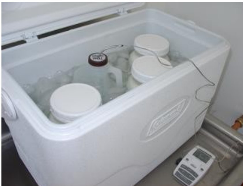
Monitor temperatures to assure effective cooling.
