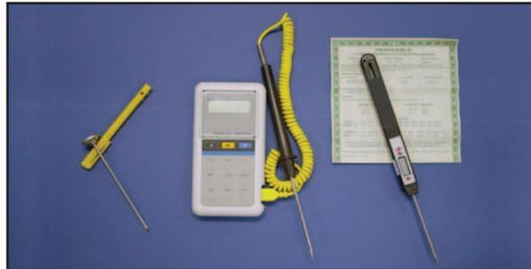
The method and frequency of calibration for thermometers will depend on the use and temperature range where the equipment is used. In the absence of manufacturer's recommendations, thermometers should be calibrated at least once a month with more frequent calibrations when the instrument is physically abused or if the readings are questionable.
