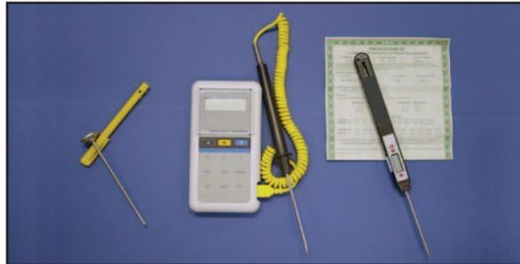
The method and frequency of calibration for thermometers will depend on the use and temperature range where the equipment is used. In the absence of manufacture's recommendations, thermometers should be calibrated at least once a month with more frequent calibrations when the instrument is physically abused or if the readings are questionable.
